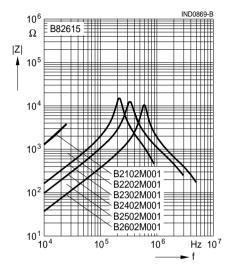
**Impedance IZI versus frequency f** measured at +20 °C, typical values
