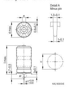
Mounting holes d = 16 mm ... 21 mm
